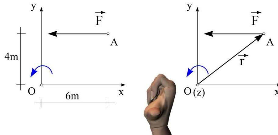
$$\vec{F} = -2\vec{i} \text{ (kN)}, \quad \vec{r} = 6\vec{i} + 4\vec{j} \text{ (m)}$$
