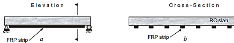
Figure 15. One-way slab strengthening, [22]
