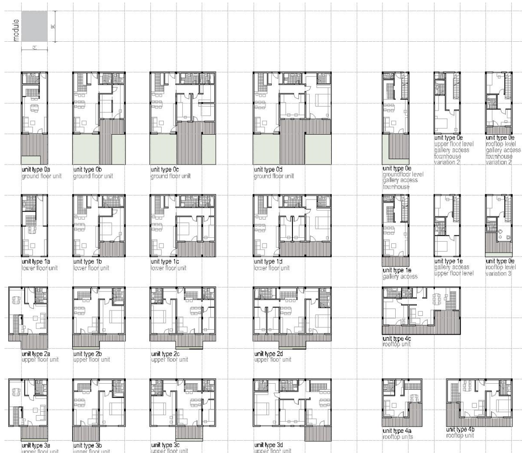
Figure 4. Variation of units' spatial layout in Mix-Mesh model of LRHD housing Source: author
