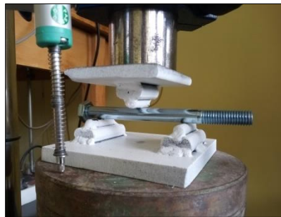
Figure 7. Bolt testing using three-point bending test
