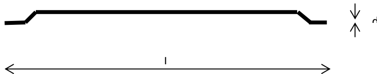
Figure 1. Shape of hooked-end steel fibers
