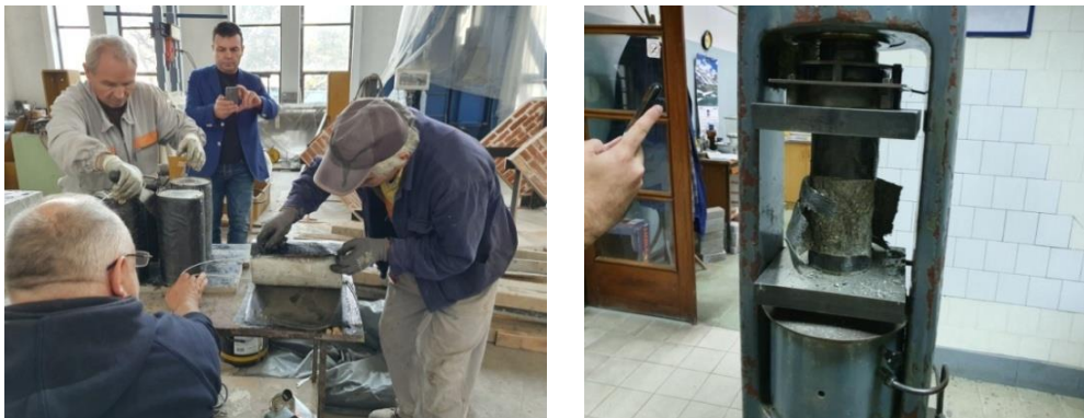
Figure 5. Preparation of strain gauges on concrete cylinders.
