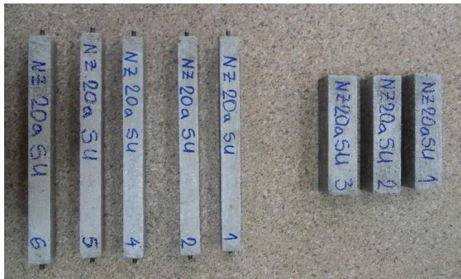
Figure 1. Unmolded NZ20a mortar bars and prisms
