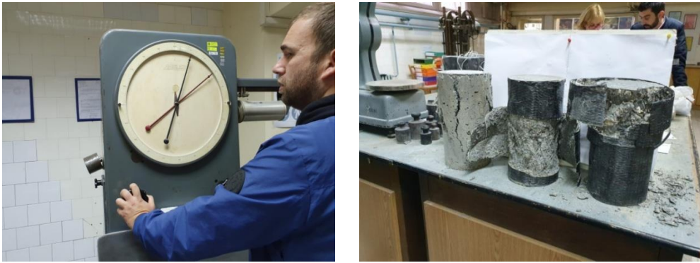
Figure 6. Testing of compressive strength of concrete for the three series
