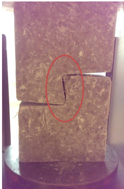
Figure 6. Typical Failure mode for SCFRC “Z”-shape specimen
