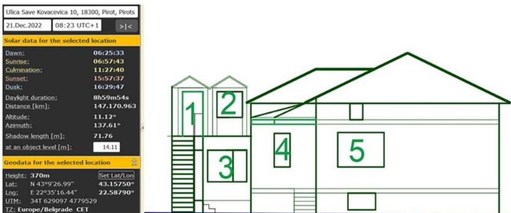
Figure 5 South-East facade of Building 1 and Building 2 at CP-1831 Pirot City, with facade opening marks that were analyzed and data on inclination and azimuth angles of solar radiation incidence
