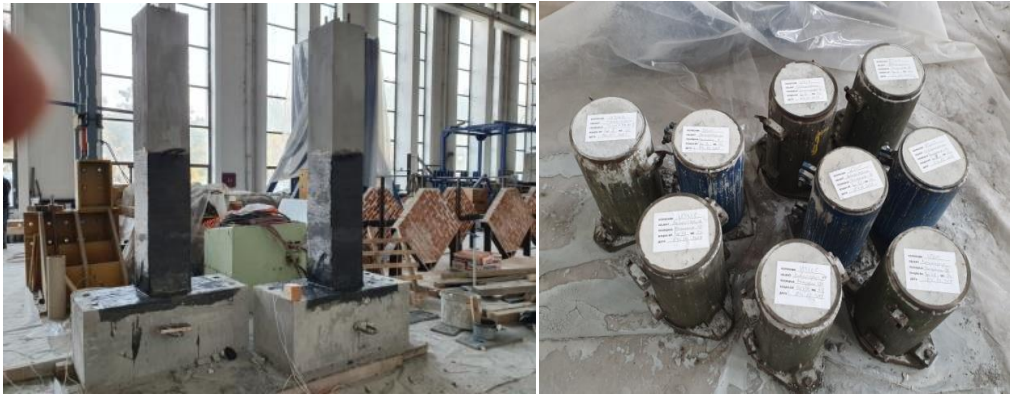
Figure 4. Photos of taken trial concrete specimens from Model M1 and Model M2
