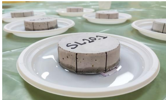
Figure 1. Determination of mortar capillary water absorption
