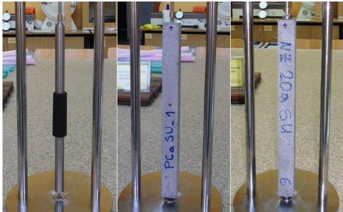
Figure 3. Determination of the length change of mortar bars due to exposure to the sulphate solution
