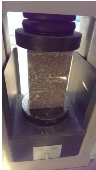
Figure 3. “Z”-shape specimen during testing
