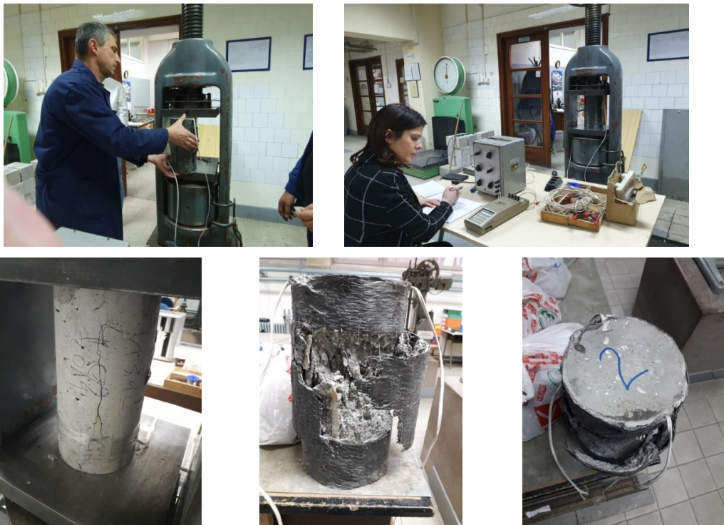
Figure 8. Testing of the static modulus of elasticity of all three series.
