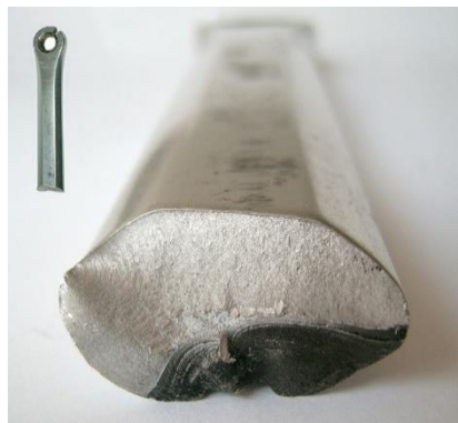
Figure 6 – Failure due to fatigue [14]
