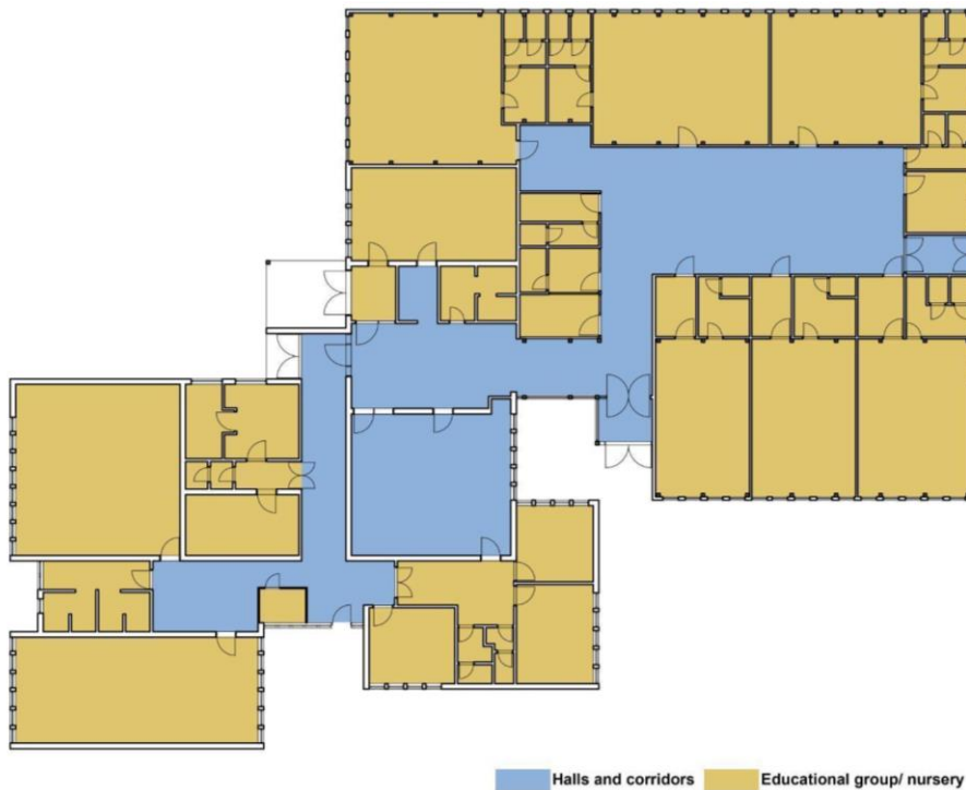
Figure 2. Presentation of the informal area boundaries on the Bubamara kindergarten floor plan (Author: S. Ickovski)
