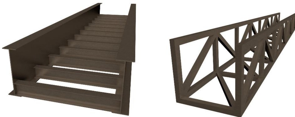
Figure 1. Half-through bridge types
