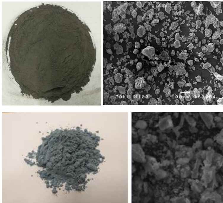
Figure 1. Photo and SEM display of used binder materials: FA (up), VEM (down)
