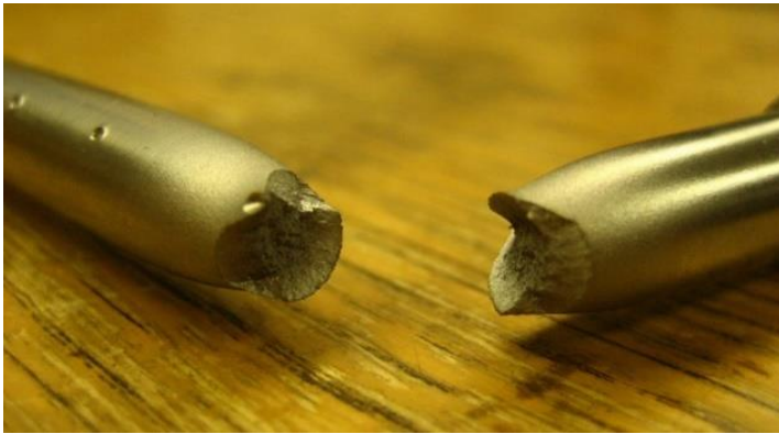
Figure 2 – Plastic fracture that indicates local thinning and irregular fracture surface [10]
